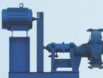
OVERHEAD IN-LINE MOTOR MOUNT
